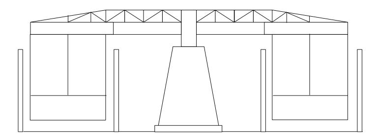
Entire Pad MUST be flat, NO Grade Deviation or Fall (NO 1% GRADE FOR DRAINAGE)
